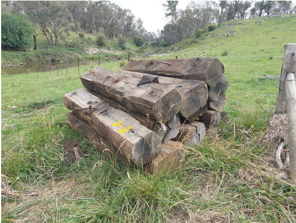
Figures 2 & 3 : Bridge corbels, 2.2m long
