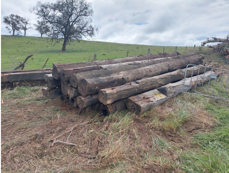
Figure 1 & 2 : Bridge girders, 7.6m long
