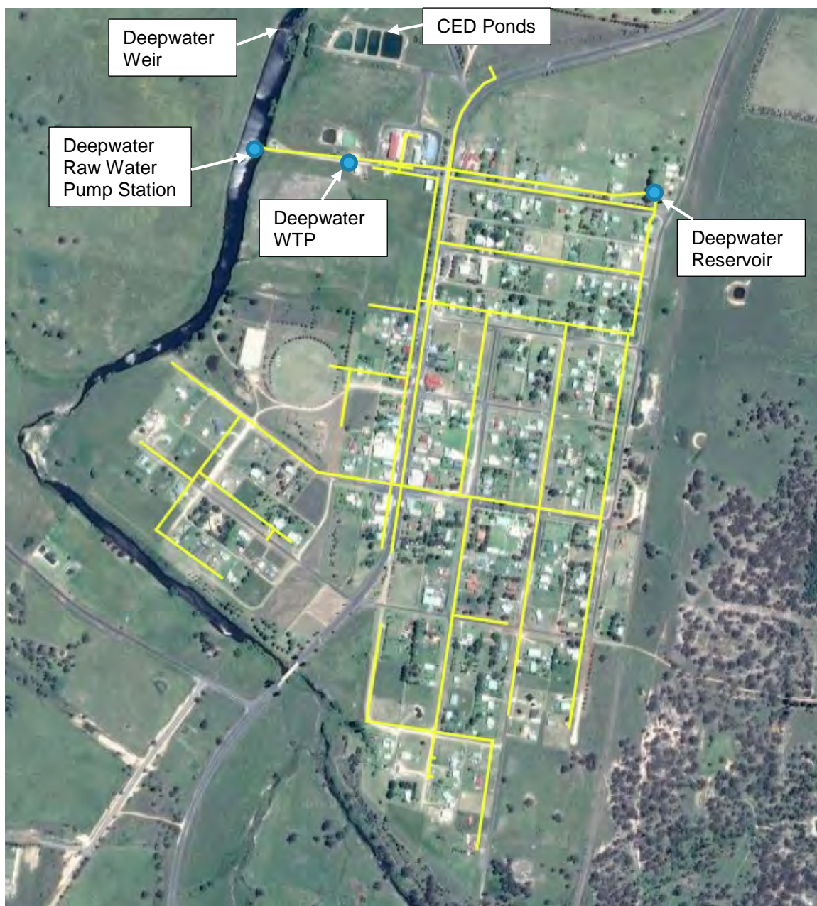
Figure 6 Deepwater Drinking Water Supply System
