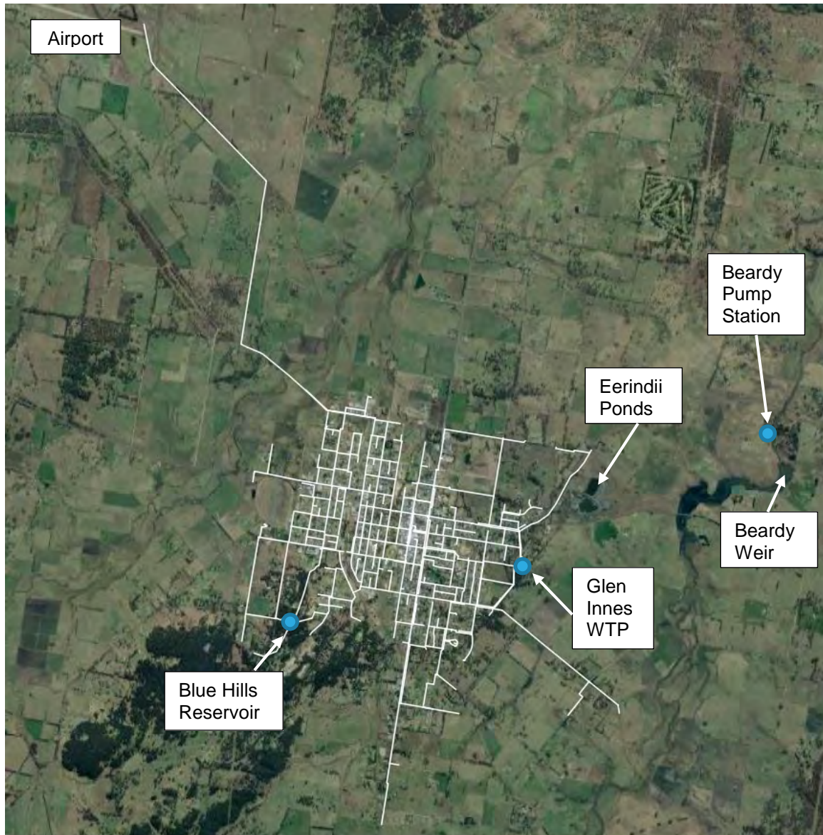
Figure 3 Glen Innes Drinking Water Infrastructure Map
