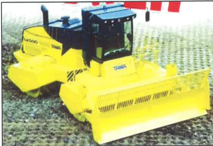
Photograph 2: A heavy, steel-wheeled Tana compactor with a Year 2005 price tag
