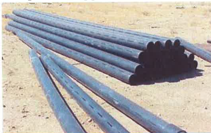
Figure 30: Slotted gas extraction pipe
