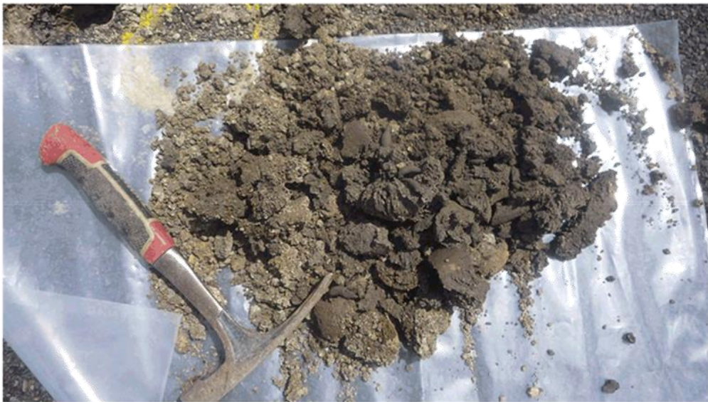
BH01 – Organic Clays Subgrade
