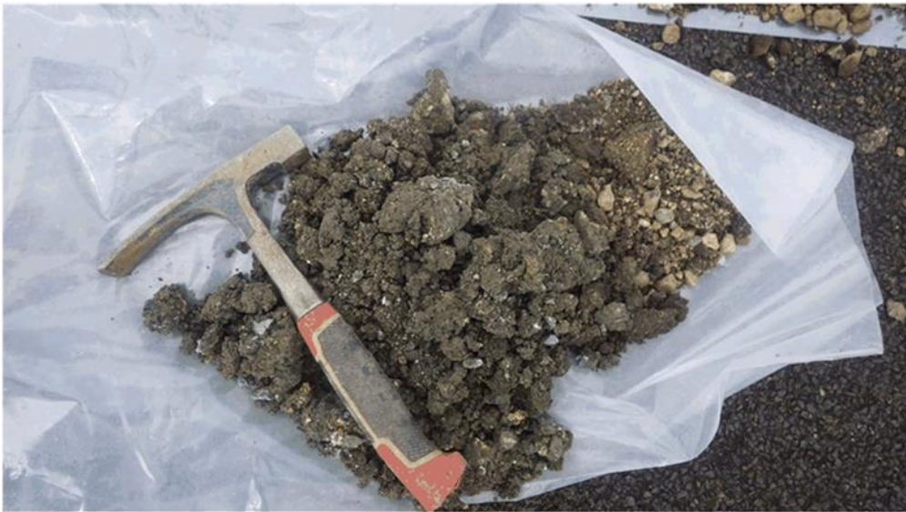
BH03 – Subgrade clay
