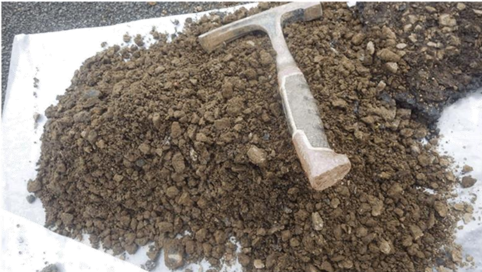
BH07 – Granular base course
