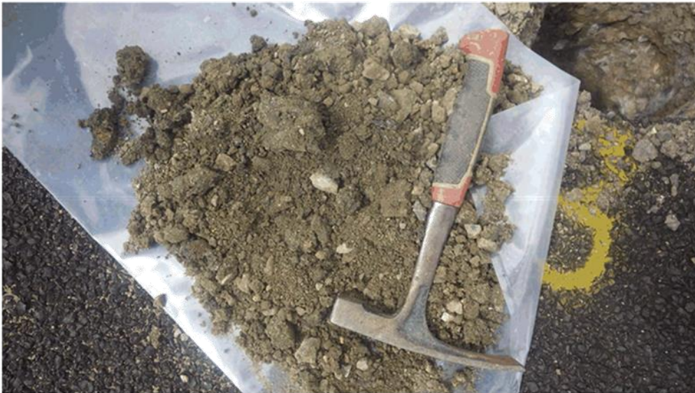
BH02 – Subgrade Clay
