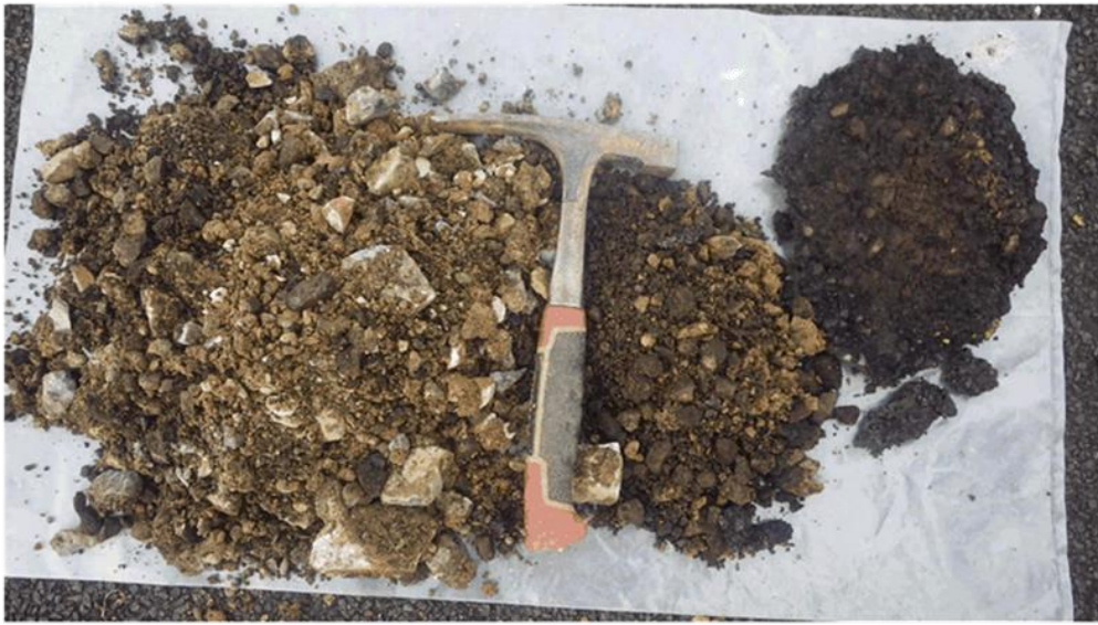
BH10 – Granular Base Layer
