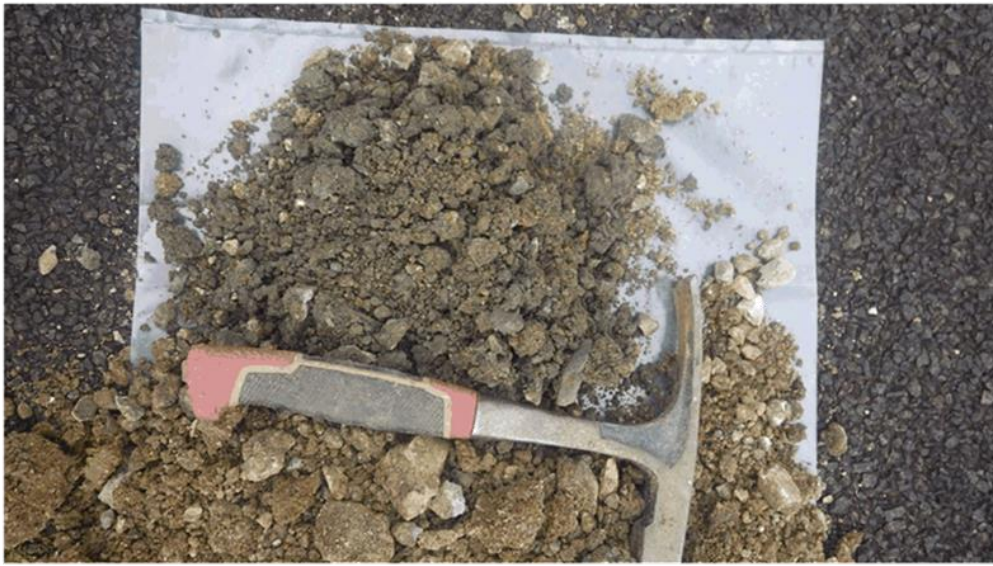
BH09 – Subgrade Clayey Sand
