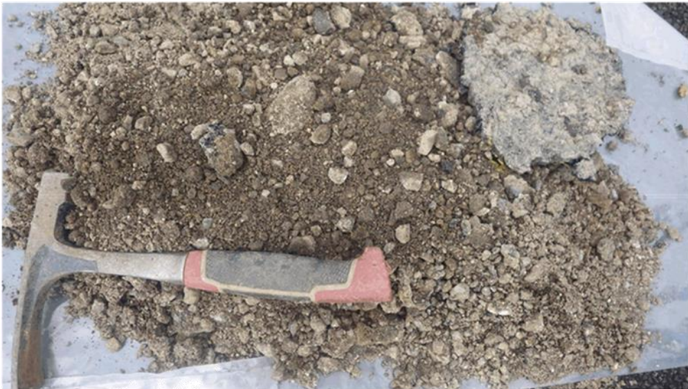
BH04 – Granular Base layer
