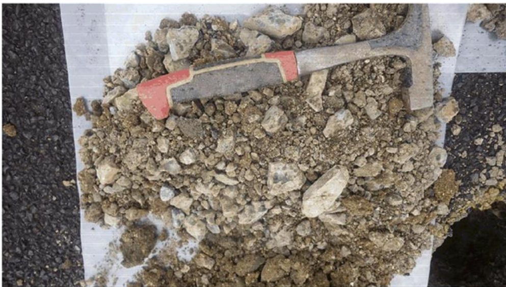
BH05 – Granular subbase
