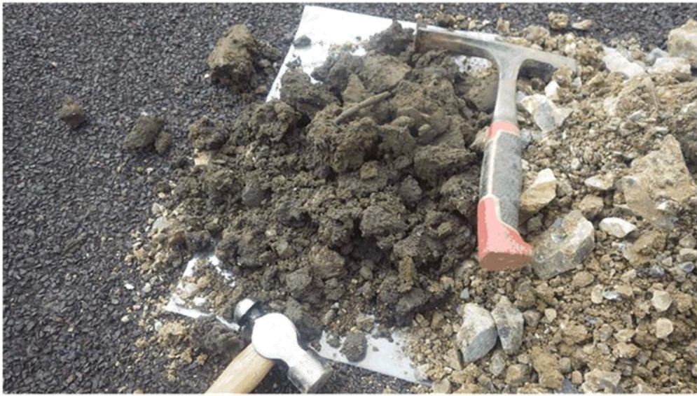
BH11 – Subgrade Organic Clay
