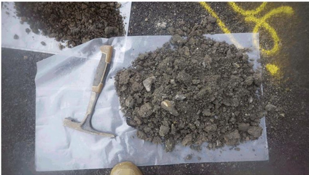
BH06 – Granular Subbase (clayey sands)
