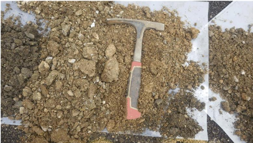
BH09 – Granular subbase
