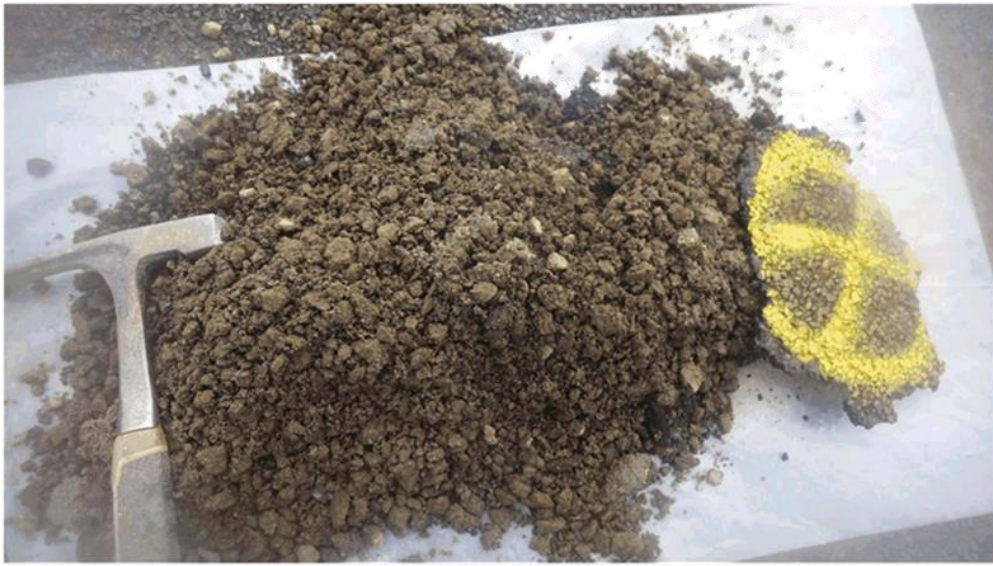
BH06 – Granular Base Course
