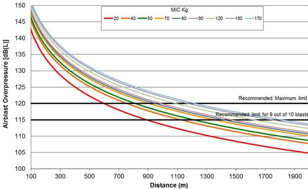
**Figure 6-2 Air blast overpressure predictions for different charge masses and distances**
