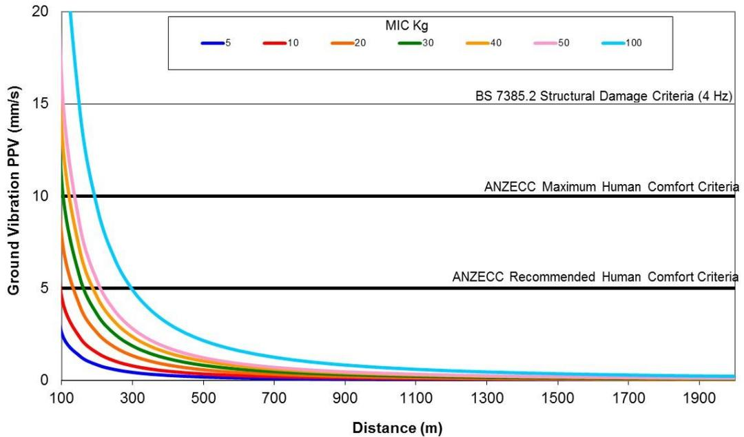
**Figure 6-1 Ground vibration predictions for different charge masses and distances**
