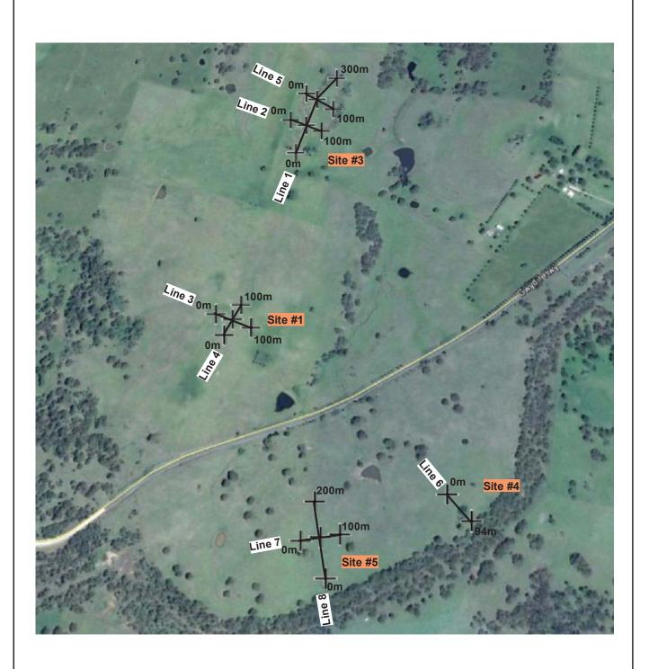
SMEC / Glen Innes Severn Council Seismic Refraction Survey "Wattle Vale" Property, Glen Innes Aerial Photo Site Plan - Seismic Lines Earth Technology Solutions Pty Ltd ABN 12 078 325 628
