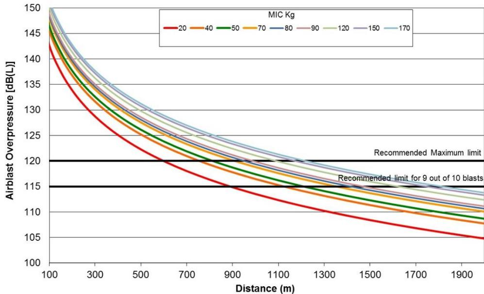
**Figure 7-4 Air blast overpressure predictions for different charge masses and distances**
