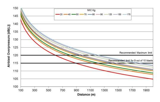
Figure 6-2 Air blast overpressure predictions for different charge masses and distances
