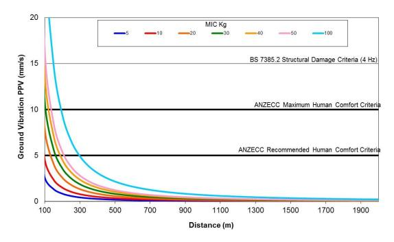
Figure 6-1 Ground vibration predictions for different charge masses and distances
