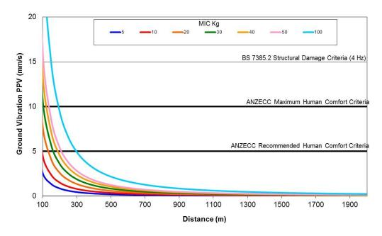
Figure 7-3 Ground vibration predictions for different charge masses and distances
