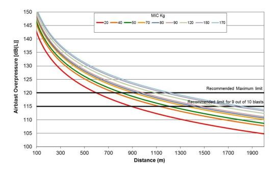
Figure 7-4 Air blast overpressure predictions for different charge masses and distances
